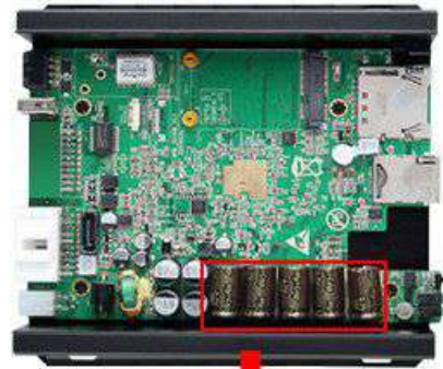
The super capacitor power the machine for 10 seconds
